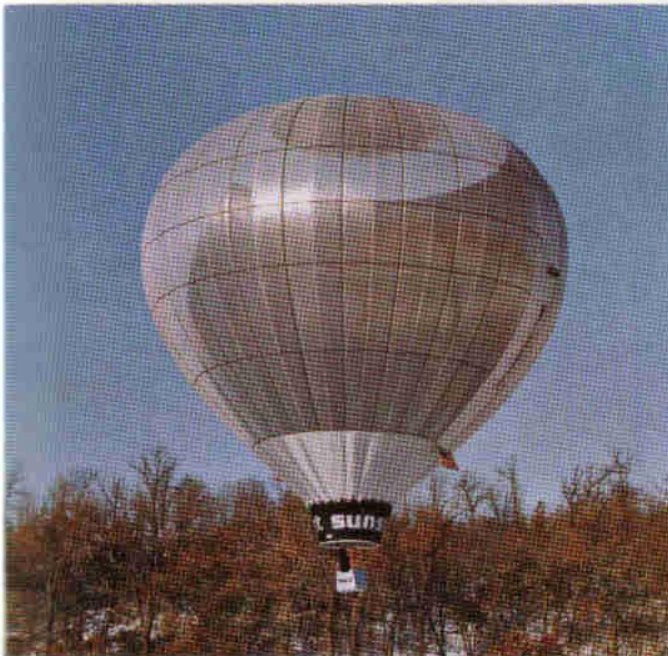
Resembling a giant parabolic antenna, the black interior of the Sunstat 's collector absorbs the radiant energy of the sun as the balloon climbs aloft on its 31-minute maiden voyage.
