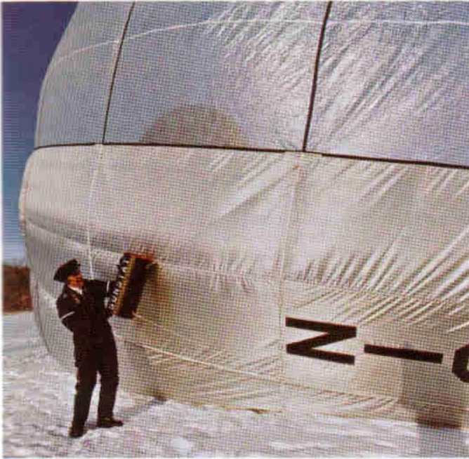
Fredrick attaches one of the electric trim motors to the Sunstat equatorial band as the balloon is prepared for its maiden voyage at Crystal Lake, Minnesota.
